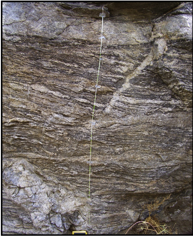
Fig. 6. Example of the method of gathering line traverse data. Green traverse in Figs. 9 and 10; total traverse length is 1669 mm. Melanosomes are marked on a ribbon taped to a subvertical, foliation-perpendicular surface. Leucosomes are represented by the intervening unmarked spaces. Field notebook (at very bottom of photo) for scale.
